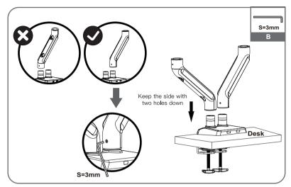
Install the lower arm to the base. Secure the arm by tightening the inside screw using 3mm Allen key.
