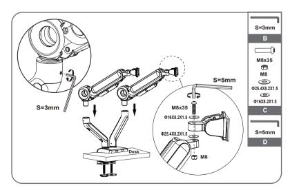
Insert the gas spring arm above the lower arm and fasten the screw in the front.
