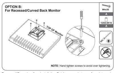
Recessed/Curved surface installation:Put 4 spacers between faceplate and monitor.Install 4 long screws through faceplate,spacers to monitor via mounting holes.Do not tighten the screws excessively or your monitor might be damaged.
