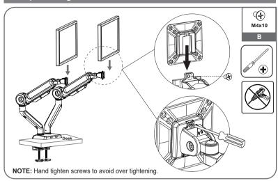
Slide the monitor onto the head of swivel arm, install the security bolt. Make sure the security bolt is installed before you rotate the monitor.
