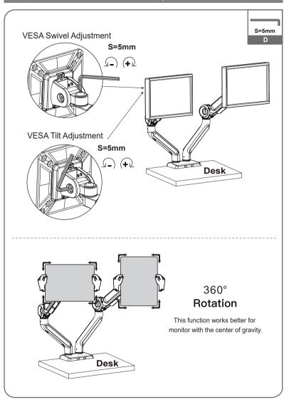
Use a 5mm hex wrench to adjust the damp for Tilt , Swivel and Rotation. Turn counter-clockwise to reduce damping and clockwise to increase damping.
