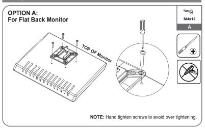
Flat surface installation:Install 4 short screws through faceplate to monitor via mounting holes.Do not tighten the screws excessively or your monitor might be damaged.
