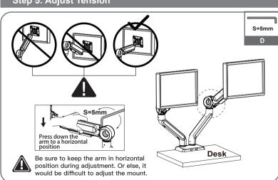
For proper functioning of this mount, depending on different weight of monitor you might need to adjust tension in the gas spring arm using 5mm hex wrench.
