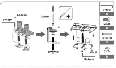
NOTE:If your desk has an existing grommet hole, remove plastic cover before installation. If there is no existing grommet hole, make a mrak on your mounting surface, and use a drill to drill a hole (10-12mm) in the mounting surface.
